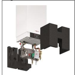
Viessmann has eliminated the need for a separate low loss header and connecting pipework for its Vitodens 200-W commercial wall boiler (49 to 150 kW) by incorporating the header in a new pump connection set.
