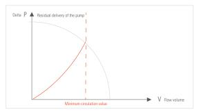
Hydro AutoControl regulates the minimum circulation quantity
