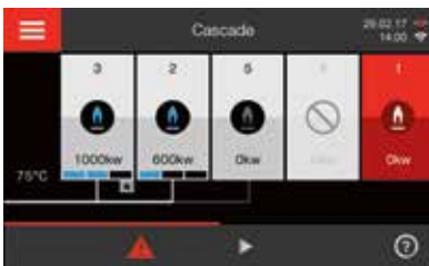
Display of the Vitotronic 300 (type CM1E). For multi-boiler systems with up to 8 boilers
